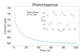
**mG-FET Photoresponse.** Au/Ferrocenyl Undecanethiol//Graphene on top of Si (SiO<sub>2</sub> = 290 nm) wafers operating at  $V_{BG}$  = 10 V,  $V_B$  = 10 mV, ambient conditions and illumination of 21.5 mW led (Thorlabs MCWHF2).
